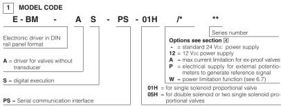
E-BM-AS digital drivers supply and control the current to the solenoid of Atos proportional valves without transducer, according to the electronic reference input signal. The solenoid proportionally transforms the current into a force, acting on the valve spool or poppet, against a reacting spring, thus providing the hydraulic regulation.
